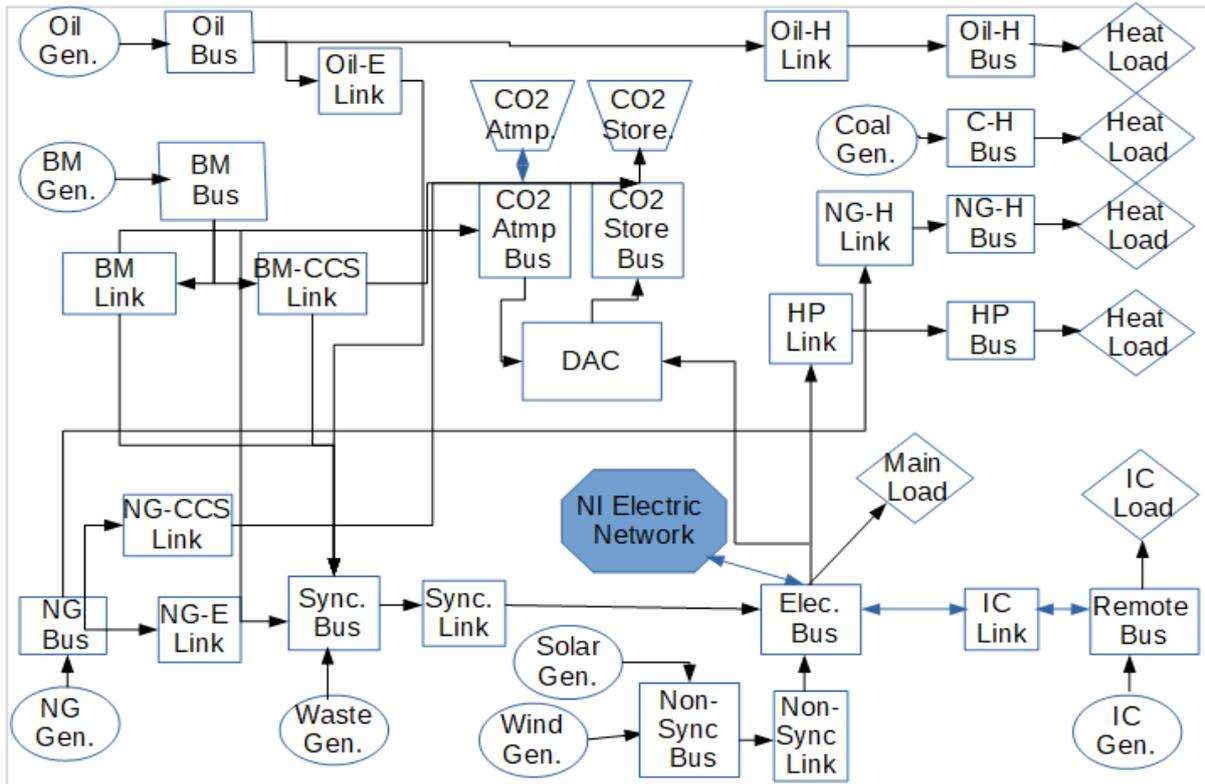
Figure 5: Electricity and Heating with CCS and DAC.
