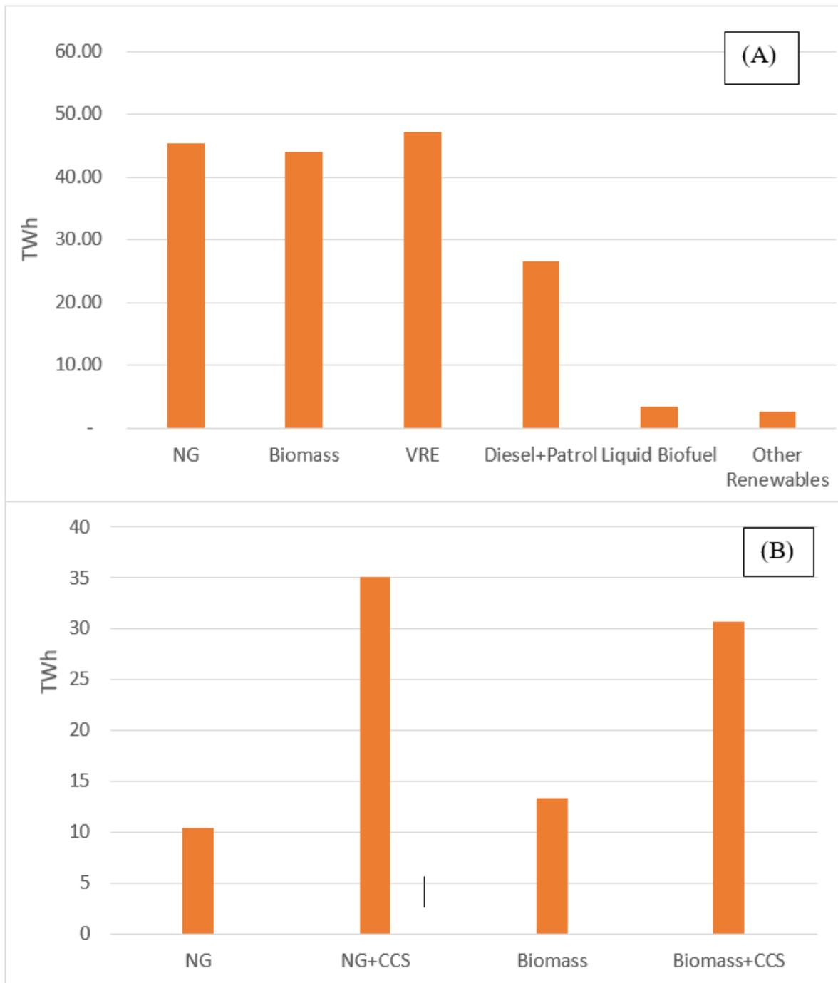
**Figure 8: (A) Required annual generation capacity to service the transport sector for the net-zero scenario; (B) NG and biomass generation breakdown to service transport sector for the net-zero scenario.**
